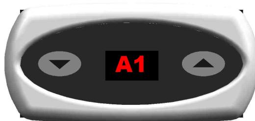
IN CASE OF PROBE SHORT-CIRCUIT THE DISPLAY SHOWS THE FOLLOWING ALARM MESSAGES:
