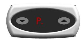
PRESSING THE INDICATED BUTTON TO INPUT A NUMBER THAT FOR THIS MACHINE WOULD HAVE THE VALUE EQUAL TO 1 THE VALUE WILL INCREASE BY PRESSING THE BUTTON DX AND DIMINISH BY PRESSING THE BUTTON SX
