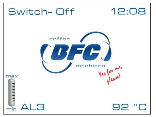
In this case it is necessary to check the incoming water connection and the gauge to ensure there is pressure. If the connection to the water supply is correct, the warning can be reset by turning the machine off and on again; the machine will start filling again until the level is reached.
