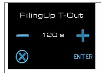
Filling Up Time-Out function; this parameter regulates the maximum water filling time in the boiler. If the necessary water level is not reached in the predefined time, a message will be shown on the display (see image below). Set the desired time in seconds using the + and - keys. Press the enter key to go to the next function.
