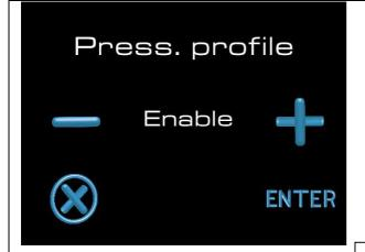
Pressure profiles function; this parameter allows coffee to be delivered with personalised pressure profiles in models equipped with the relevant kit. This function can be enabled or disabled using the + and - buttons. When this function is enabled, an icon relative to profile settings is displayed (see paragraph 3-d user manual). Press the enter key to go to the next function.
