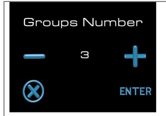
Groups Number Function; using the + and - keys set the number of groups on the machine being configured to allow its ideal operation. Press the enter key to confirm and move on to the next function.
