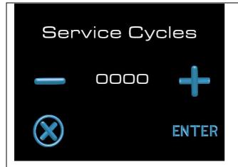
Service Cycles function; this parameter allows a number of cycles to be set, after which routine maintenance must be performed. It is set in steps of 1000 cycles. Set the desired number of cycles using the + and - keys. Once the number of set cycles has been reached, the display will show a message indicating the need to perform maintenance (see following image). Press the enter key to go to the next function.
