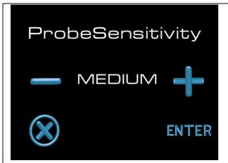
Probe Sensitivity function; this parameter regulates the sensitivity of the water level probe in the boiler. The value can be set using the + and - buttons at three different levels of sensitivity; high (suitable for water with a low mineral salt content), medium (suitable for water softened with a traditional softener) or low (suitable for water with a high mineral salt content). Press the enter key to go to the next function.
