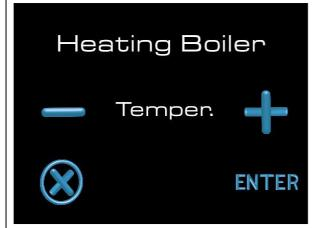
When Temperature is selected, the temperature settings menu is shown with relative PID parameters (boiler kP, boiler kI, boiler kD, Pid boiler set.) that regulate heating. It is recommended not to change the parameters in this section, as they are factory-regulated by qualified operators.
