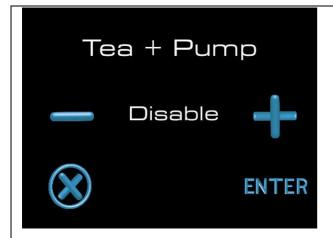
Tea with Pump function; this parameter controls water mixing for tea. If enabled, when the water is delivered, the pump is activated to guarantee more accurate and constant mixing, preventing pressure fluctuations in the water inlet system. If disabled, mixing occurs without the use of the pump. This function can be enabled or disabled using the + and - buttons. Press the enter key to go to the next function.
