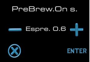
Pre-brewing values can be changed using the + and -buttons. Press enter to confirm the set value and move on to the next setting. The pre-brewing on time indicates the duration of the water spurt in seconds, used to moisten the coffee blend. The pre-brewing off time indicates the duration of the stoppage in seconds, before dosing. Once the times have been set for each dose, press the enter key to go to the next function.
