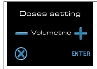
Dose Setting function; this parameter makes it possible to work with doses managed by the volumetric counter, or with timed doses. Use the + and - buttons to change the selection. Set Volumetric to programme doses, determining the quantity of water delivered through the volumetric counters. Set Timer to programme doses, establishing the interval between the start and stoppage of delivery. Press the enter key to go to the next function.
