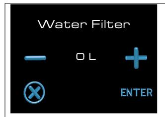
Water Filter function; this parameter allows the amount of water in litres to be set using the + and - keys, after which the softener needs to be regenerated. Once the set amount of water has been reached, the display will show a message indicating the need to regenerate the filter (see following image). Press the enter key to go to the next function.
