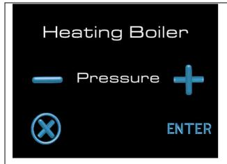
Heating Boiler function; this parameter allows boiler heating to be managed by way of a pressure gauge (Pressure) or temperature probe (Temperature).
