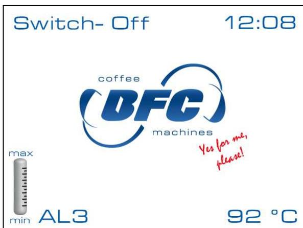
If the following screen appears during water filling in the boiler, the set boiler water filling time has been exceeded. The machine therefore needs to be restarted.
