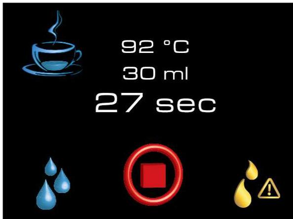
If the indicated symbol appears during delivery, the water filter needs to be changed. This operation must be performed by qualified personnel.
