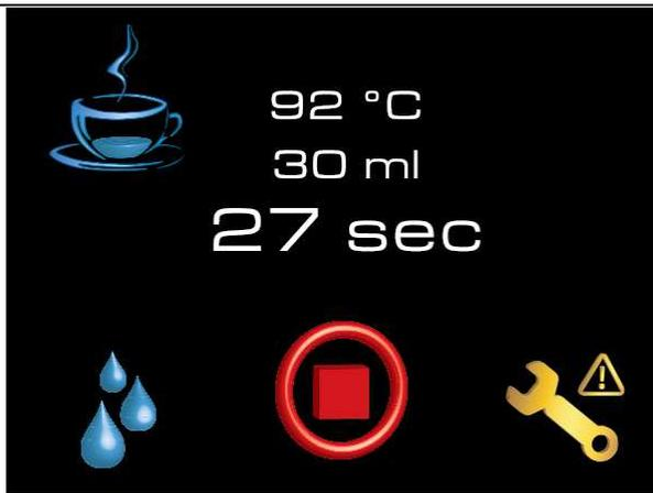
If the indicated symbol appears during delivery, maintenance needs to be performed on the machine. This operation must be performed by qualified personnel.
