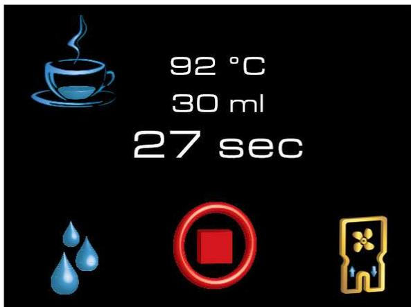
If the indicated symbol appears during delivery, pulses are not being received by the volumetric counter for the activated group, because it is either interrupted or blocked. Run a completely empty dose and check that the dosing process is correct; in this case the problem may be caused by too finely ground coffee. If the problem persists, contact the technical help centre.
