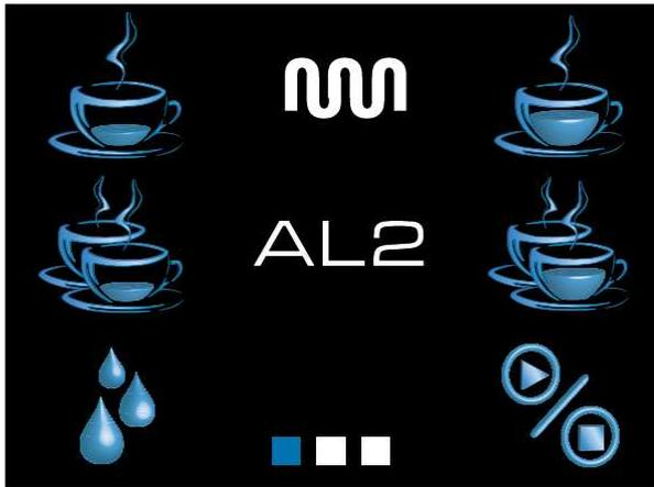
If the message AL2 appears on the indicated screen, the temperature probe in the relevant group boiler is short-circuited. Contact the technical help centre to solve the problem.
