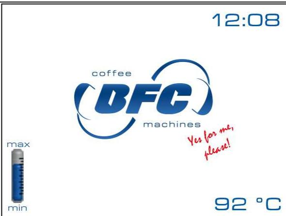
When the machine starts, it is in standby. The machine also goes into standby if none of the displays are used for more than 5 minutes. When in standby, the display shows the time, the temperature of the group to which the display refers (only in multi-boiler models) and the level of water in the boiler. Press any point on the display to go to the next screen (see paragraph 2)
