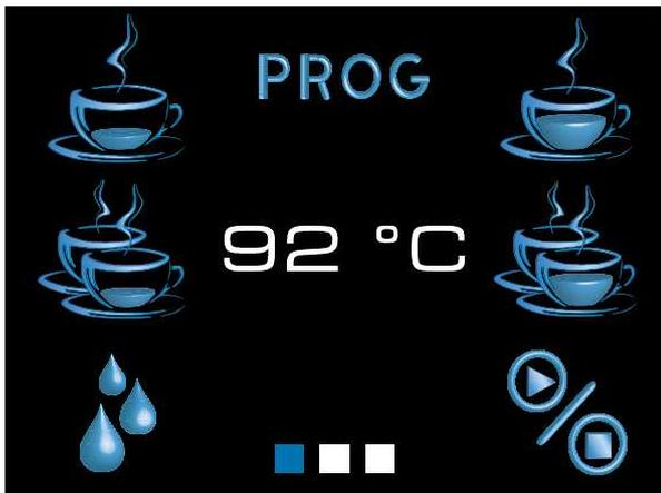
When the dose programming icon is pressed the following screen appears. It is now possible to programme the amount of coffee for each dose; to change and memorise coffee dose quantities, press the desired key and start delivery; when the desired amount of coffee is reached press the Stop button to stop delivery and memorise the data.
