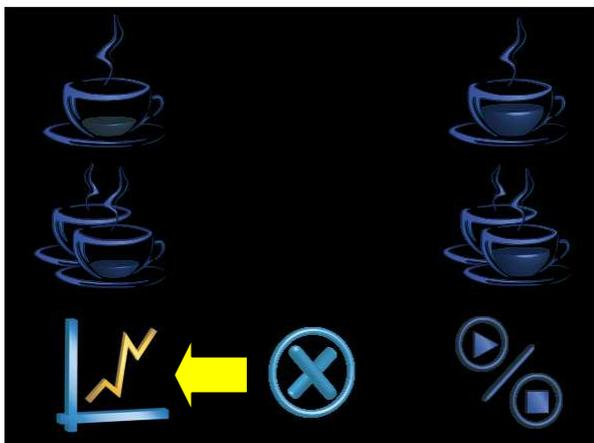
Press the indicated icon to disable the pressure profiles relative to the group from which the operations are being performed; the dose icons will darken to indicate that they have been disabled. In this way, traditional delivery will be enabled.
