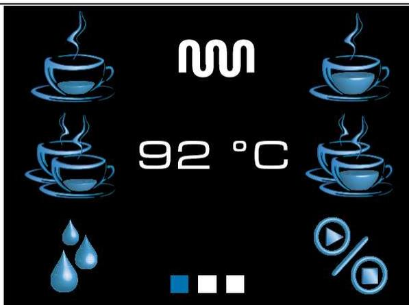
This screen displays the icons for espresso, double espresso, hot water, long coffee, double long coffee doses and continuous delivery. The resistor icon for the running group, the real time group temperature (only in multi-boiler models) and the selected screen is then displayed. To go to the next screen (see paragraph 3) press the centre of the display.
