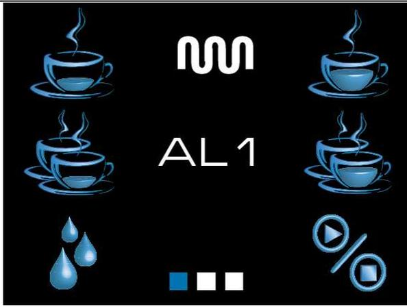
If the message AL1 appears on the indicated screen, the temperature probe in the relevant group boiler is disconnected or interrupted. Contact the technical help centre to solve the problem.
